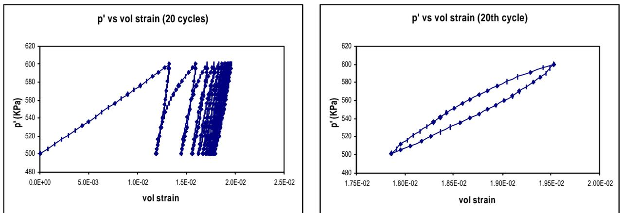
Figure 3. Mean normal effective stress against volumetric strain.
