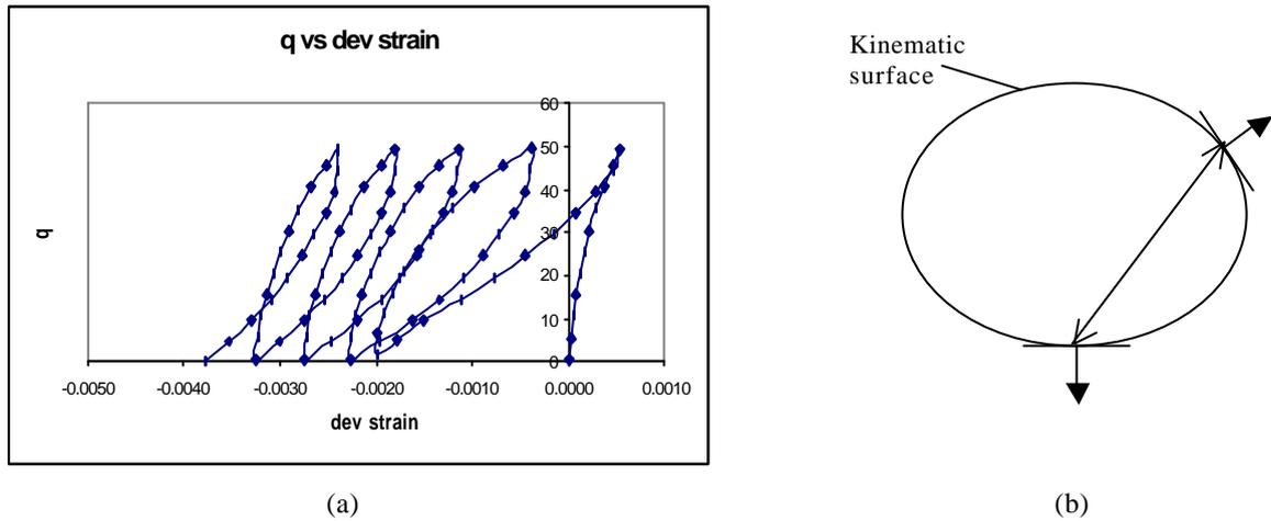
Figure 4. (a) Increasing negative permanent shear strain and (b) position of load cycles relative to the kinematic yield surface.
