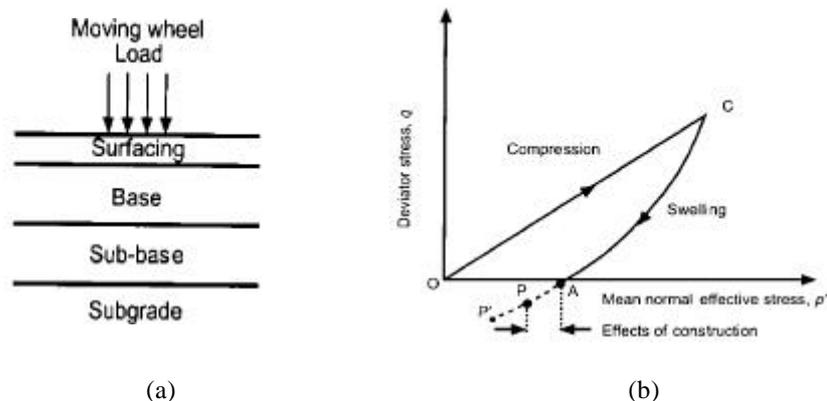
Figure 1. (a) Cross section of a pavement and (b) typical stress history of a pavement.
