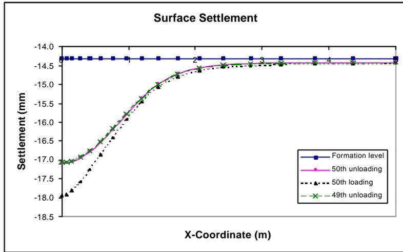
Figure 2. Permanent settlement of a pavement after 50 cycles.
