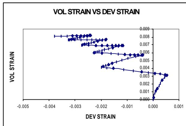
Figure 5. Volumetric strain against deviatoric strain
