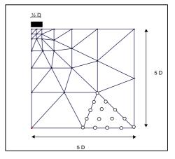
The finite element mesh for the strip footing (plane strain) is shown on right. Normalised plots of collapse load against settlement are shown below.
